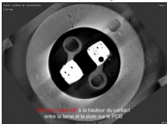
EasyTom 160 - Voxel size : 4µm - Acquisition on whole part (40x30x10mm) Pollution by corrosion products at the blister/PCB interface : Contact impossible
